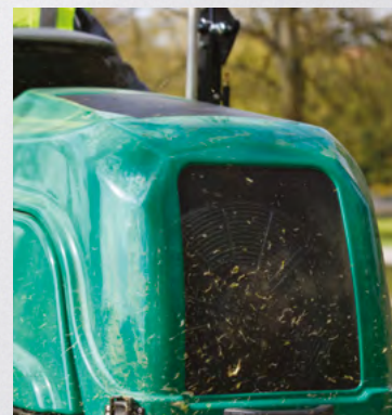
Easy-access engine bay & reversible cooling fan
